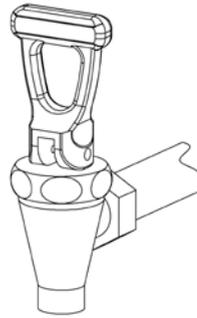
The discharge tap is closed when the lever points upwards.
