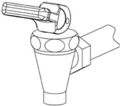
The discharge tap is opened when the lever is pressed down.
